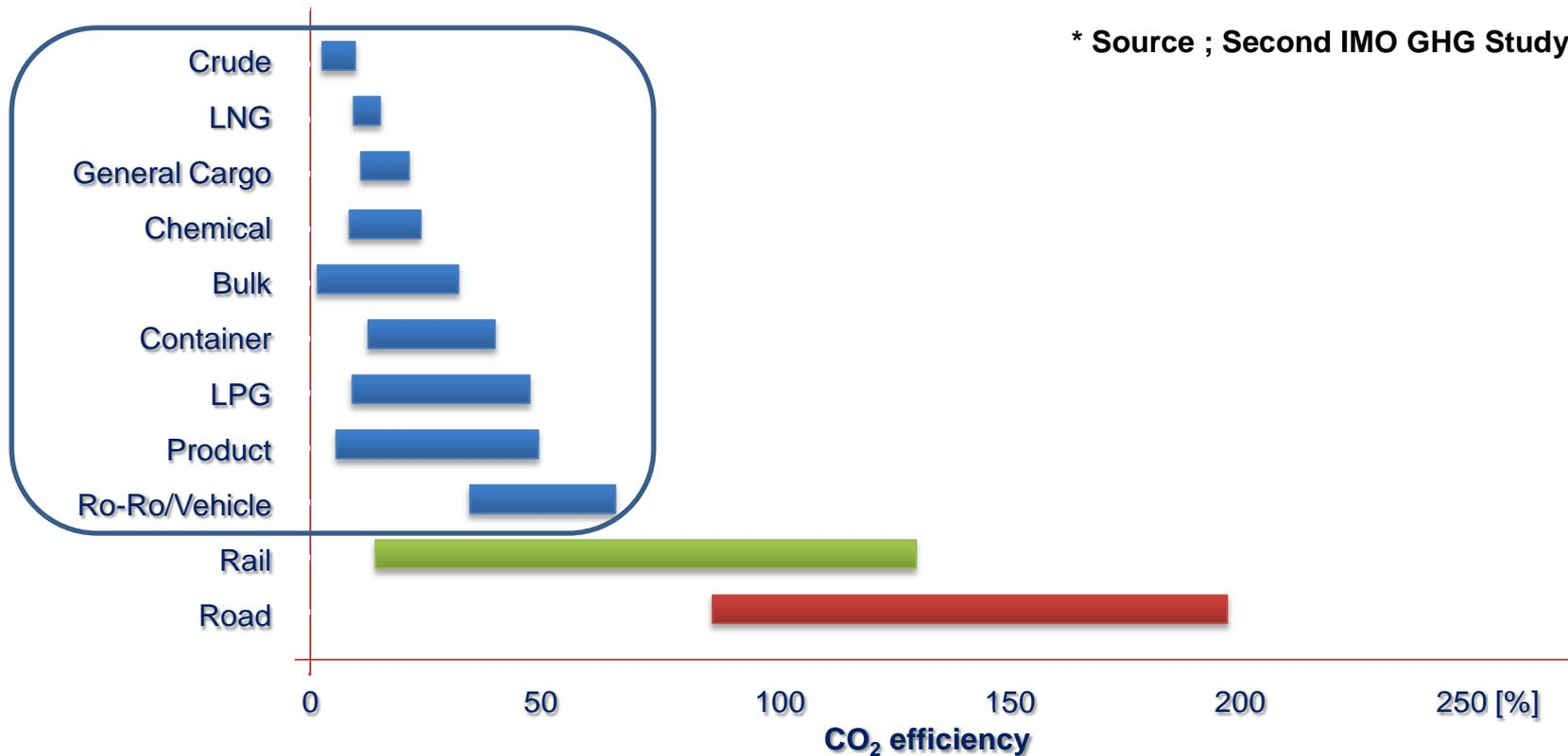
$CO_2 \text{ efficiency} = CO_2 / (\text{tonne} * \text{kilometre}) \approx \text{Fuel consumption}$
