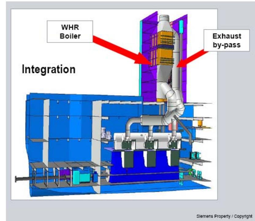
Shaft generator and WHRS of Siemens
